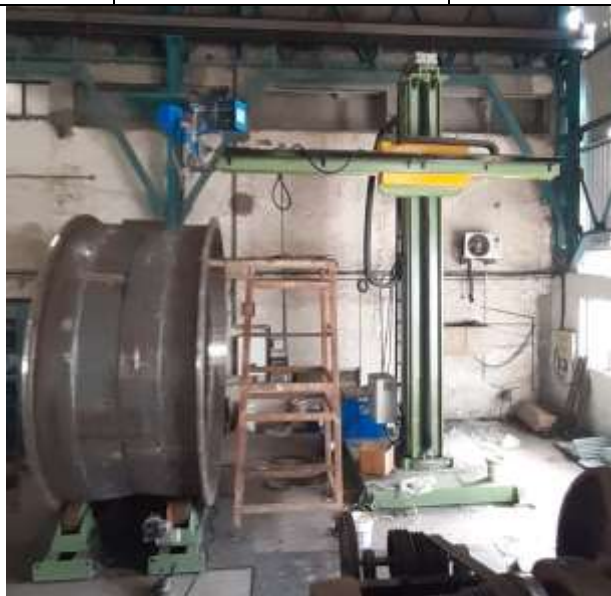
CU-BUILT- Make column Boom welding Machine
